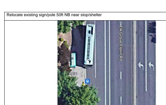
Replace rolled curb sidewalk with 6' x 45' vertical curb sidewalk/gutter Repave 30' x 45' area adjacent to new curb/gutter to centerline Secure ROW at 9231 Elk Grove-Florin Rd (APN 127-0160-048) Construct 4' x 16' pad behind new sidewalk
