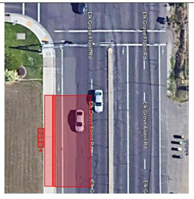
Existing stop location is in intersection; move sign/pole 60ft NB to farside of Camden Dr Construct new 8' x 60' sidewalk, vertical curb/gutter Repave 20 x 60' area adjacent to new curb/gutter to centerline
