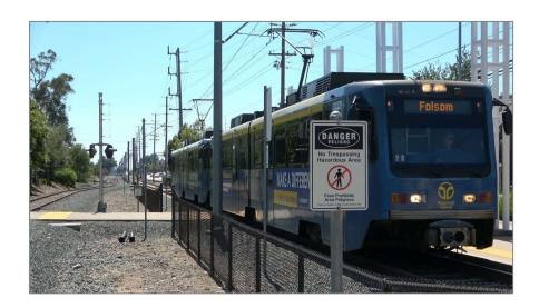
Capacity – Each of the new Siemens s700 cars has 58 seats, so a 2-car train will have 116 seats, which is sufficient for the existing peak load of 73 passengers as well as the projected future peak load of 64 passengers, although seasonal and day-to-day variation are expected to increase the peak load above 64 passengers on many days.
