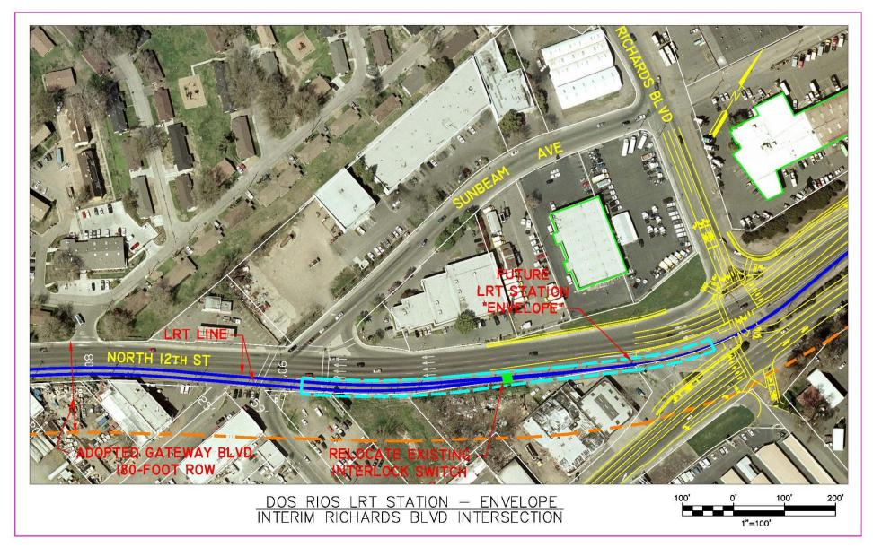
Figure 4-2: Dos Rios-Area LRT Station Envelope (Site D) and Richards Boulevard Interchange Concept
