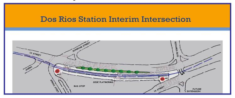
Figure 2-1 illustrates a concept layout for Site D with the "Interim Intersection" concept for the extension of Richards Boulevard. The station is located between Sproule and Richards with side platforms, bus connectivity via Sproule and strong art elements.
