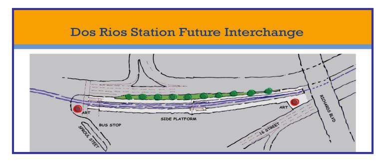
Figure 2-2 above illustrates a concept layout with the "Proposed Interchange" for the Richards Boulevard extension for Site D. This station concept has similar design elements as the previous concept with the main difference being the grade separation. Because of the overpass at the north end of the platform, an ADA-compliant means of directly accessing Richards Boulevard to the north would be required for pedestrians to access Richards Boulevard and the CIHC if it is located in this area.
