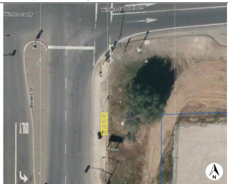
Stop ID: 574 3 on, 4 off Priority: 4 SB Winters St & Grand Ave (MB) Secure ROW at GRAND AVE (APN 252-0092-037) Construct 4 x 16' concrete pad behind existing sidewalk
